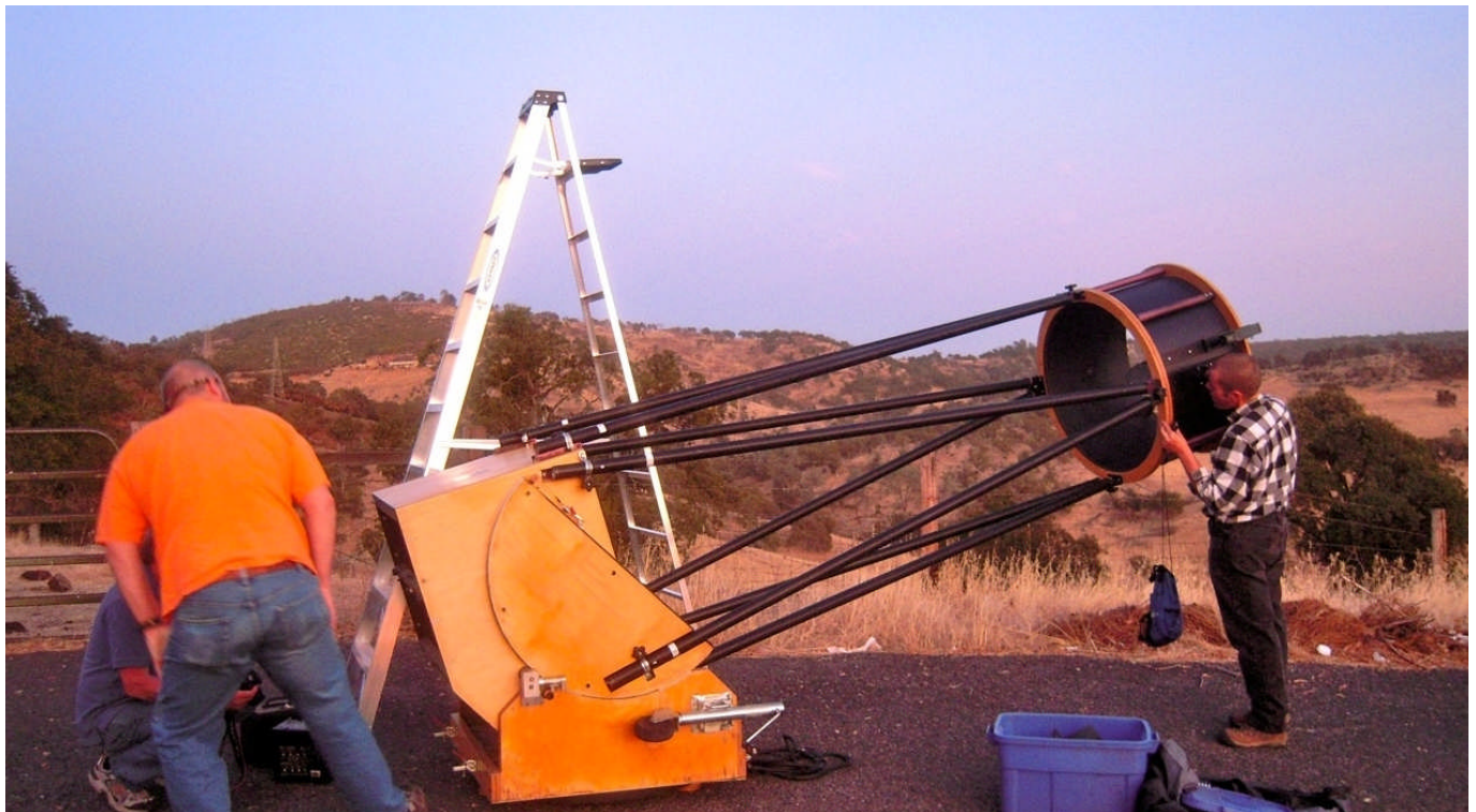
Bret's new baby — a 30" f/4.5 Dobsonian (Some baby!)
